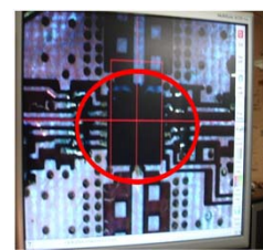
Final placement with pressure and/or temperature
