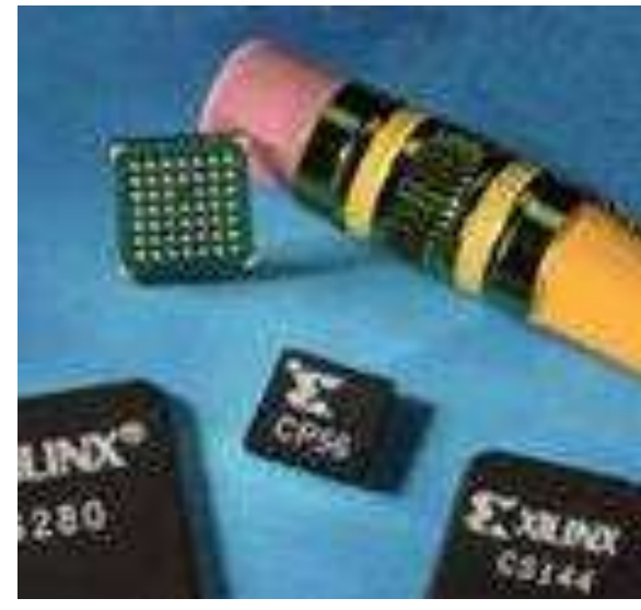
CSP : Chip Scale Package
